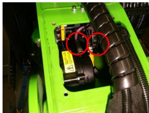
Figure 17: Leaf chain pulley greasing points in the front end of the upper boom.
