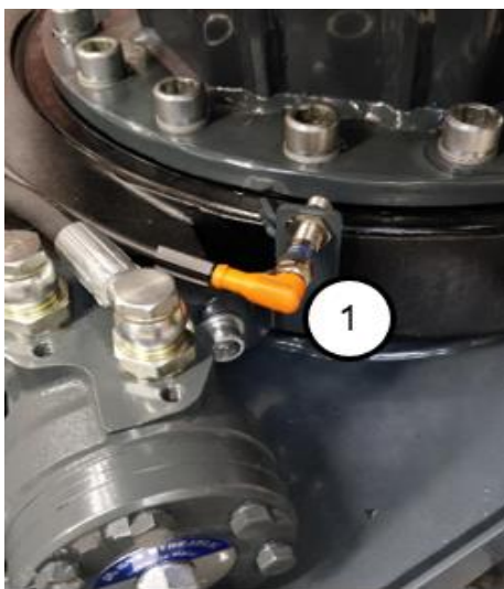
Figure 26 Slewing angle sensor
