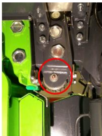
Figure 16 Telescoping chain pulley grease nipple
